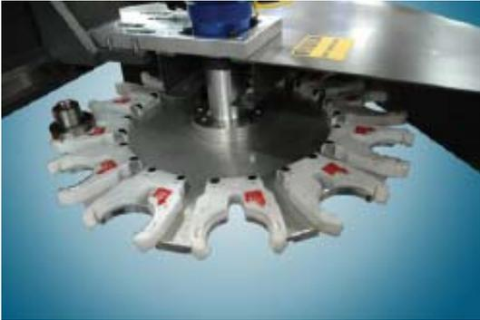
Order an optional 12-position rotary tool changer for 5000 Series machines. MultiCam optimized this accessory for bidirectional rotation. It takes the shortest route to help reduce tool change time. All ATC systems come standard with automatic tool calibration. Tool change routines built into the controls simplify integration with your favorite CAM software. An automatic tool changer solution will help reduce job time, improve accuracy and reduce setup errors.
