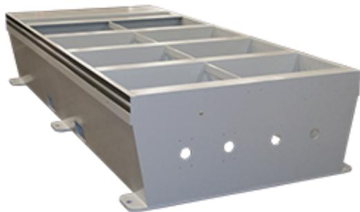
MultiCam welds, stress relieves and precision machines the one-piece 5000 Series steel-plate base frame. It features 0.5" thick side plates and 2" bar stock to support the X-axis linear bearings. One-piece construction provides a very accurate and smooth cutting system while reducing installation time greatly. It essentially removes the possibility for installation errors that could affect the system's performance and accuracy.
